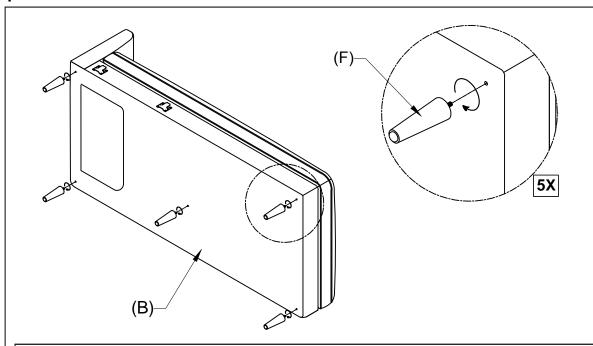
Zip cover on the bottom of Chaise (B) closed. Align Legs (F) with the corresponding pre-threaded holes on the bottom of Chaise (B) as shown. Screw legs in clockwise until they are secure.
