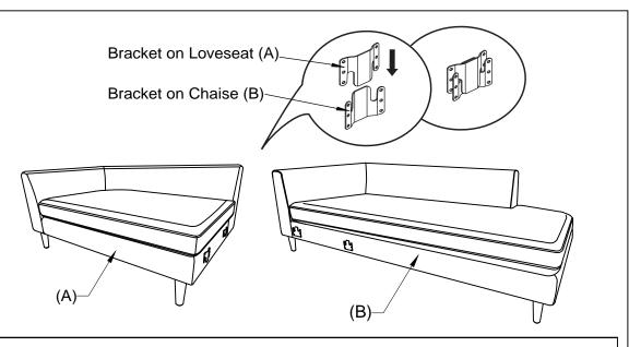
Carefully stand the Loveseat (A) and Chaise (B) assembly upright. Using a second person to assist you, carefully slide the pre-installed bracket on Loveseat (A) into the bracket on Chaise (B) as illustrated above. Once both brackets have engaged to each other, press down firmly on Loveseat (A) to secure the assembly.
