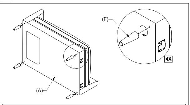
Zip cover on the bottom of Loveseat (A) closed. Align Legs (F) with the corresponding pre-threaded holes on the bottom of Loveseat (A) as shown. Screw legs in clockwise until they are secure.
